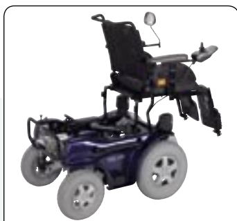
Assise amovible Facilite les interventions techniques.
